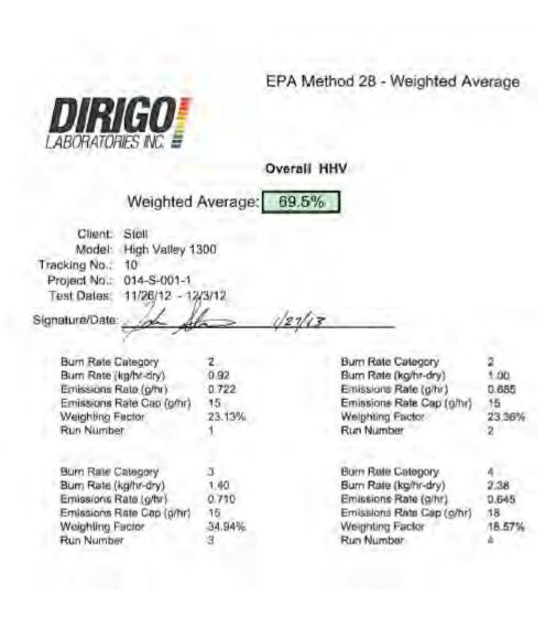
Figure 1: Overall Weighted Average Efficiency (HHV)
