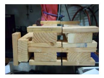
Figure 9: Fuel Load -Side View
